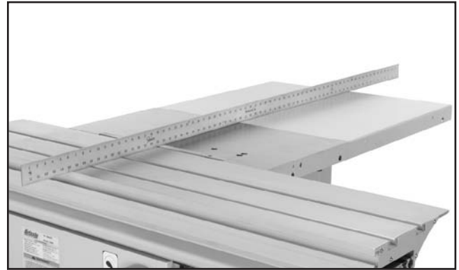
Figure 11. Extension wing mounted and adjusted evenly with the cast iron table.
